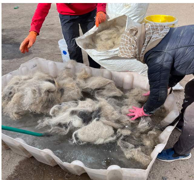
Shredded goat hair being dipped in borax solution to make it insect repellent.
